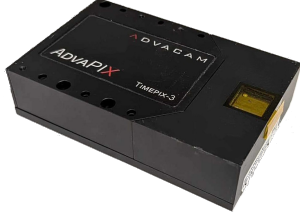
Figure 1: AdvaPix Timepix3 detection module. Figure 2: Schematic representation of sensor event readout.
