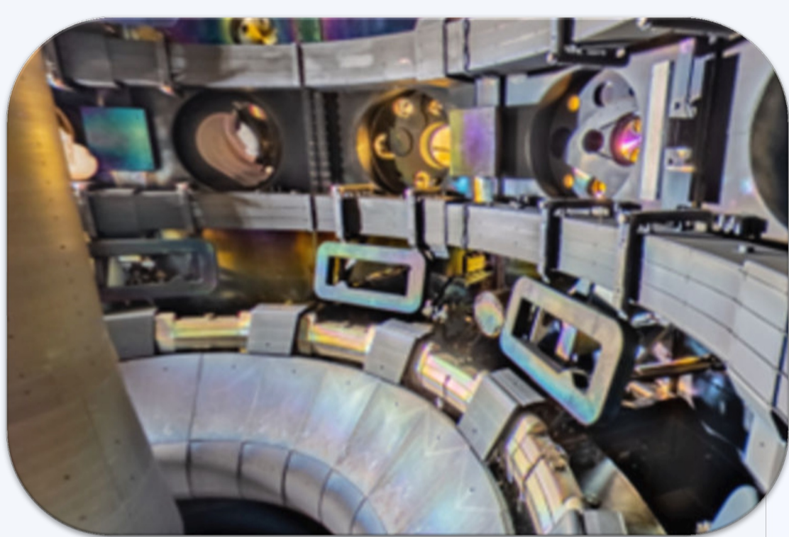
Figure 1: The Interior of the Mega Amp Spherical Tokamak (MAST) Upgrade. The plasma facing components are constructed of carbon. Credit: UKAEA
