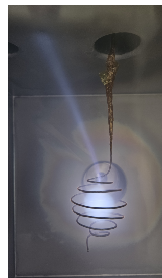
Figure 4: A test version of a fusor cage in argon.
