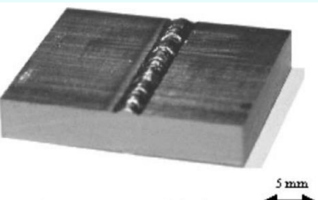
Joining of V-4Cr-4Ti by Gas Tungsten Arc and laser welding methods were demonstrated. Optimisation of the Post Weld Heat Treatment was made by optimising precipitation in weld metals [3]
