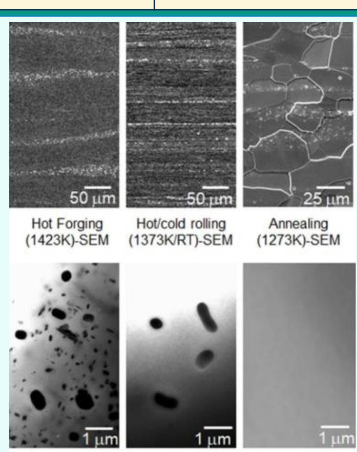
Evolution of microstructure with temperature: Precipitate formation during the fabrication process of NIFS-HEAT [1]
