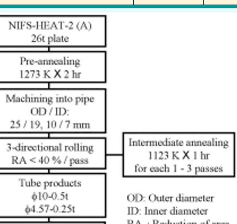
Tube forming process flow for high purity, low activation V-4Cr-4Ti alloy [2]
