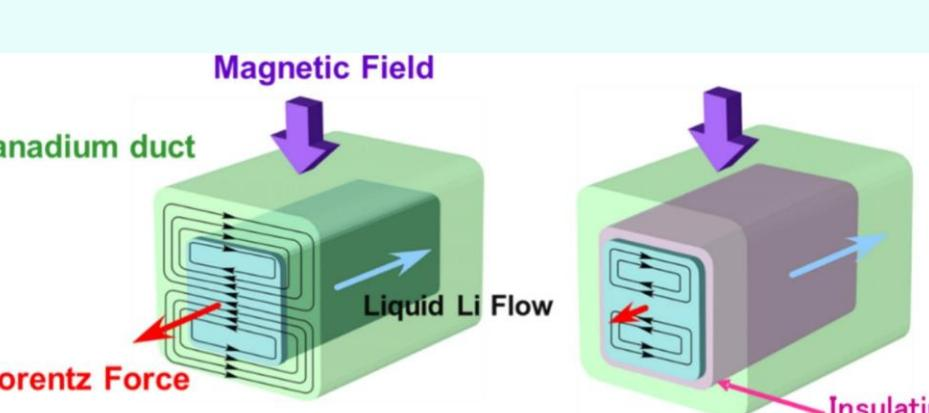
Schematic illustration of MHD (Magnetohydrodynamic) pressure drop (left) and the role of insulator coating (right) when electrically conductive coolants [1]
